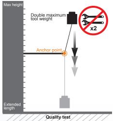
· The retractable tool lanyards are developed according to KING TONY standard. The steel lanyards are tested by double maximum weight and dropped from height. Product quality is approved.
